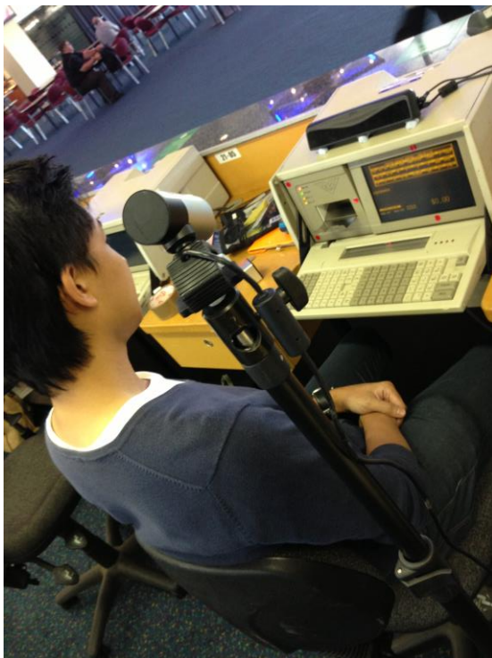
Using a Tobii X1 Light Eye Tracker during contextual inquiry
